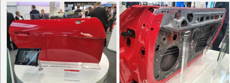
〈Fully Carbon Fiber Door〉
